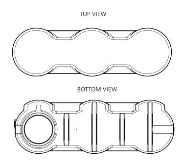
OVERFLOW CAN BE FITTED AT EITHER END
