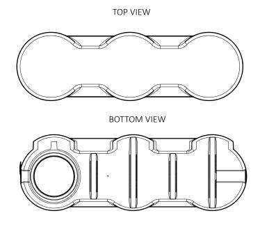
OVERFLOW CAN BE FITTED AT EITHER END
