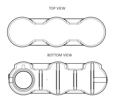
OVERFLOW CAN BE FITTED AT EITHER END
