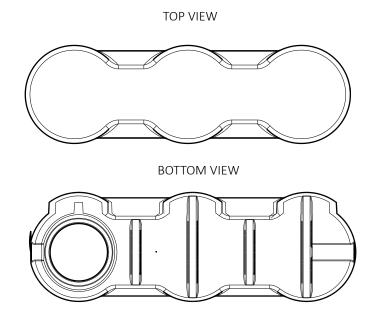
OVERFLOW CAN BE FITTED AT EITHER END
