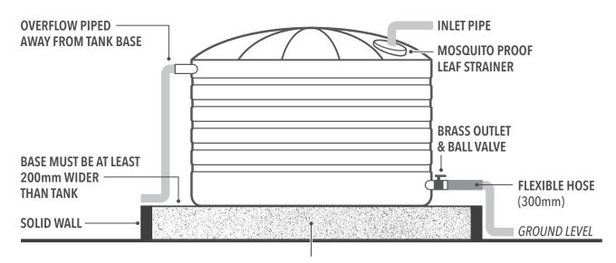
SOLID, LEVEL BASE OF CEMENT OR CONSOLIDATED FILL (RETAINED)
